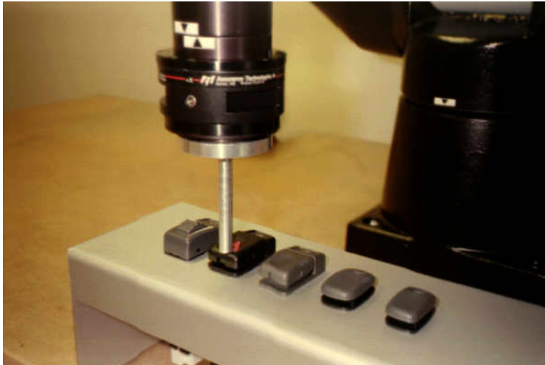
Figure 6.d. The pin tool used to press the push button switches.
