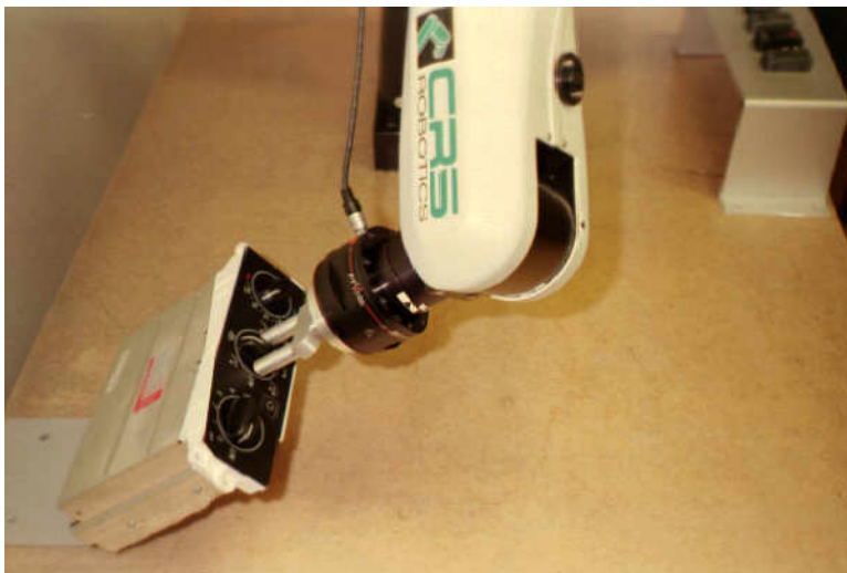
Figure 6.e. The fork-shaped tool used to turn rotary switches.
