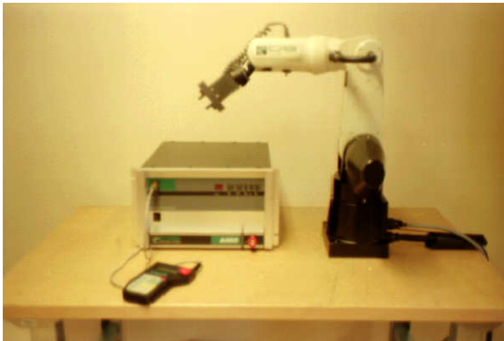
Figure 3.a. The robot system A465 from CRS Robotics Corporation.
