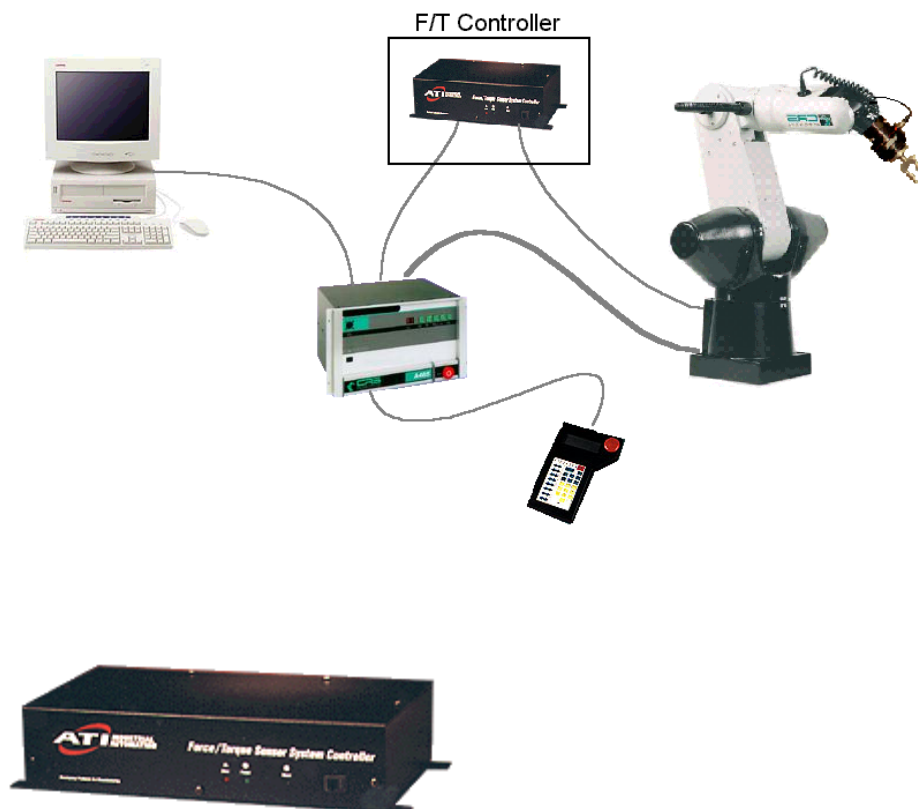
Figure 4.c. The primary function of the F/T controller is to convert analog strain gage signals from the transducer to digital Cartesian force and torque components.
